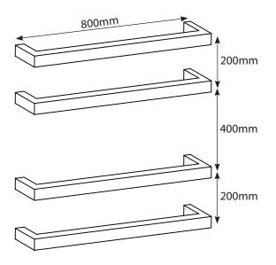
The supplied fixing bracket allows for the above configurations. If more than 5 bars are used an additional fixing bracket will be required.
