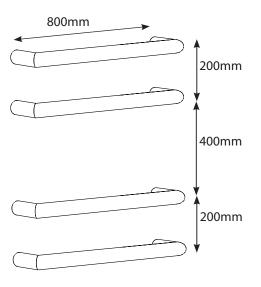
The supplied fixing bracket allows for the above configurations. If more than 5 bars are used an additional fixing bracket will be required.
