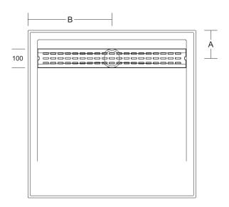
The Barossa polymarble shower base has a modern low-profile and is self-supporting. It features a 304 grade stainless steel channel grate and there are tile flanges on all sides.
