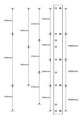
Option 1: 2, 3, 4 or 5 rails at 200mm intervals (centre to centre) Option 2: 2, 3 or 4 rails at 250mm intervals (centre to centre) Option 3: 2 or 3 rails at 300mm intervals (centre to centre) Option 4: 2 + 2 rails at 200mm intervals with a 400mm gap (centre to centre)
